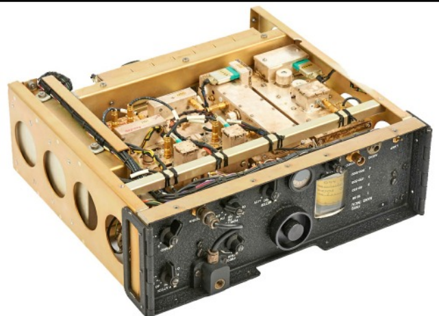
Bottom view of Radio Receiver SRR-8 showing the tuner assembly that housed four separate RF tuners.
