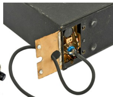
The AC power unit was housed in a compartment located at the rear of the receiver, accessible through a door of the case.
